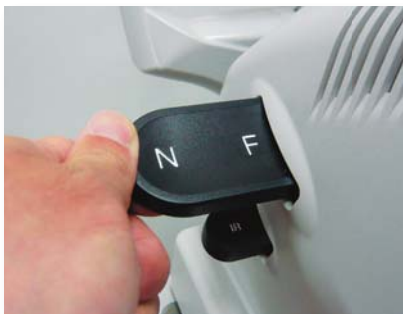
Pull in / out the RF filter selector
